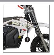
The vehicle identification number 1 is stamped into the right side of the steering stem.
