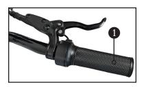
The throttle grip 1 is located on the right side of the handlebar. Rotation of the throttle engages the motor and the amount of rotation is related to engine power.
