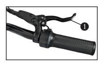
The right hand brake lever 1 is located on the right side of the handlebar.
