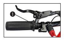
The start button 1 is located on the left side of the handlebar.
