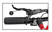
The left hand brake lever 1 is located on the left side of the handlebar.
