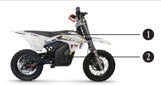
A rechargeable lithium-ion battery 1 is installed in the vehicle. The lithium-ion battery supplies the electric motor 2 with voltage. The lithium-ion battery is slid into the frame and secured in place.
