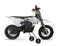
The battery **1** and the electric motor **2** are air-cooled.
