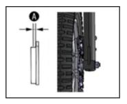
Check the brake pads for minimum thickness
