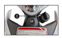
The ignition switch 1 is located to the right rear of the upper triple clamp.
